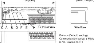
Bottom View A: Dip Switches Set communication speeds and S-No. (first digit). S-No. (station no.) Switch . Sets S-No. (last digit).
