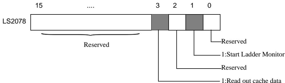
Bit 1:Turning this bit ON starts the Ladder Monitor. The Ladder Monitor menu will not appear.
