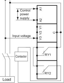
Connect the input between terminals V1-COM, V2-COM, V3-COM depending on the input voltage
