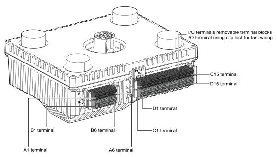
The figure shows the pin assignment of the terminal blocks:
