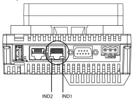
Do not confuse the RJ45 Ethernet connector with the RJ45 serial interface.
