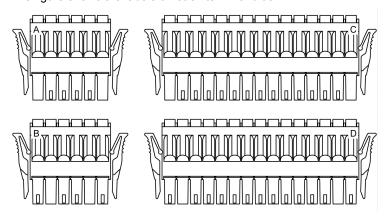
**NOTE:** Appearance of the connectors are the same but are different. Check the label and pin position of each connector before connecting.
