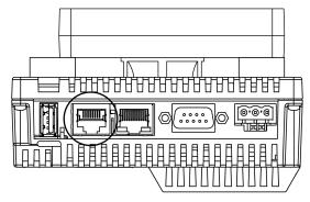
Do not confuse the RJ45 serial port with the RJ45 Ethernet interface.
