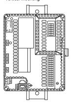
**NOTE:** Keep adequate spacing for proper ventilation to maintain an ambient temperature between 0...50 °C (32...122 °F) for horizontal installation and 0...40 °C (32...104 °F) for vertical installation.
