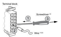
Use the following procedure to connect the wires to the terminal blocks:
