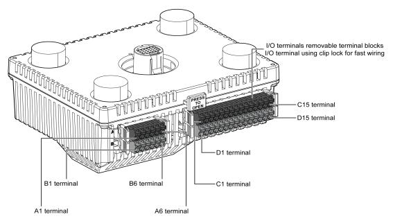
The figure shows the pin assignment of the terminal blocks:
