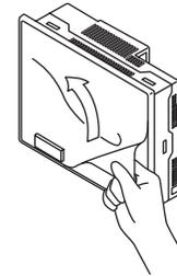
1) Remove the old protective sheet from the GOT holding the lower right corner, and clean the GOT surface.
