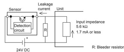
$$R(k\Omega) < 1.7(\text{mA}) / \text{Leakage current}(\text{mA}) - 1.7(\text{mA}) \times 5.6(k\Omega)$$
