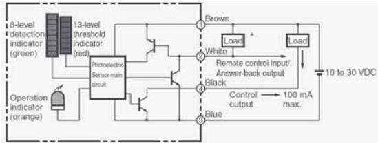
[Connector Pin Arrangement]
